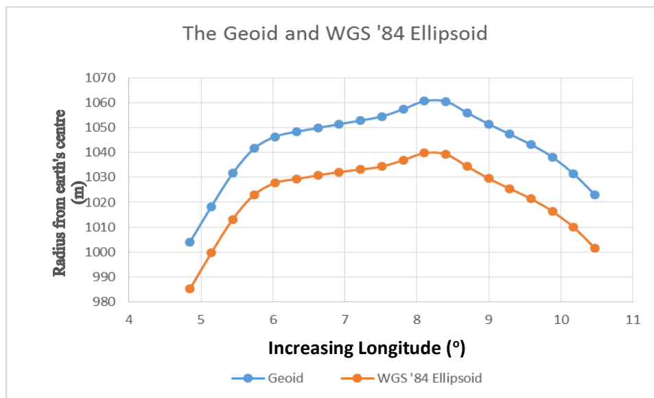
Figure 11(a): Geoid and Ellipsoid at Latitude 5° (note that a base value of 6376940 m has been removed)
