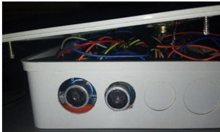
Figure 6. Packaging of the device revealing the ultrasonic sensors
